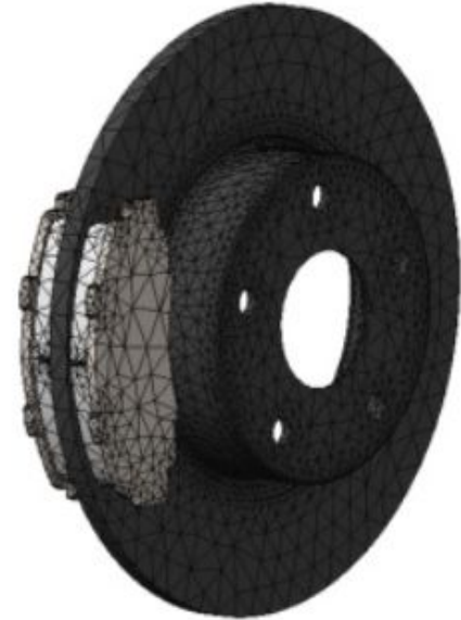
Figure 9: Full disc and pad used in simulation test [6]
